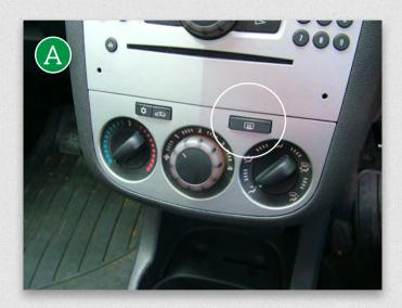
Some demisters are on a timer and switch off automatically. Some demisters have to be switched off after the screen has cleared.
