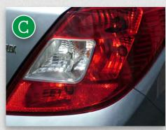
If one of the indicator lamps on one side is out the remaining lamps will flash quicker. If a rear indicator lamp is out following vehicle will not know your intention is to change position. If a front indicator lamp is out oncoming vehicles will not know your intention is to turn off a road or cut across their path.
