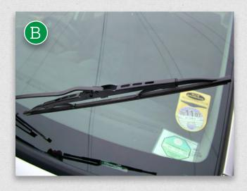
Tears on the wiper blade can produce smears on the wind screen resulting in poor vision. Tears can also lead to damage on the screen resulting in the need for a new windscreen.
