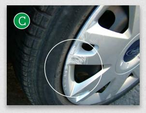
When a tyre with a damaged sidewall heats up a blow out can occur.
