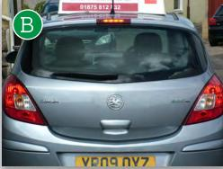
All brake lights must be operational. Faulty brake light bulbs need to be replaced straight away. If following vehicles cannot see brake lights they will not know that you are braking to slow your vehicle. Some vehicles have combined brake and tail lights. This means one bulb with two filaments, one for the tail light and one for the brake light.
