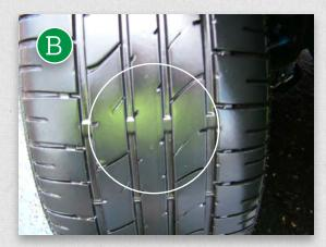
Less tread means less grip. In wet conditions this could lead to loss of control or aquaplaning
